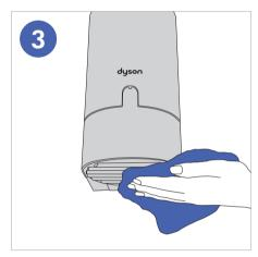
REGULARLY clean air inlets on base of motor bucket (under sink). Ensure plughole in sink is free from blockages so water can drain freely.
