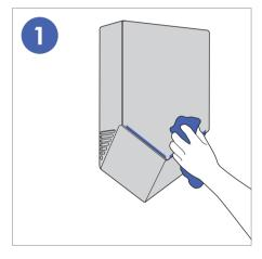
Wipe all surfaces with a soft and non-abrasive cleaner, including the air inlets on the side of the machine.
